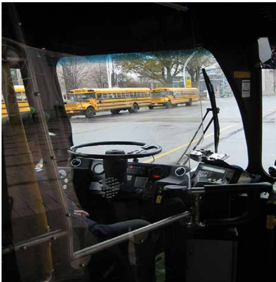
Picture 7.1: Glass barrier between driver and passenger as used in Canada
