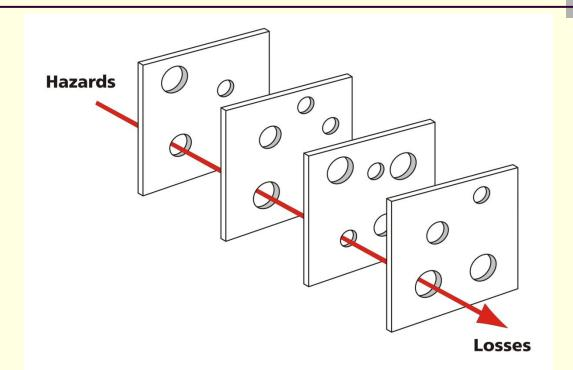
The Swiss cheese model of accident causation illustrates that, although many layers of defence lie between hazards and accidents, there are flaws in each layer that, if aligned, can allow the accident to occur.
