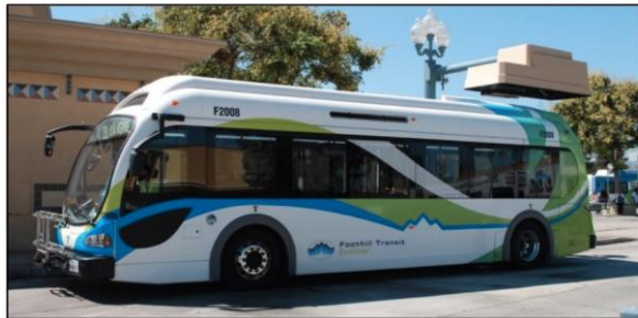
BEB parked at the charging station. The building that houses the chargers and equipment is on the left.
